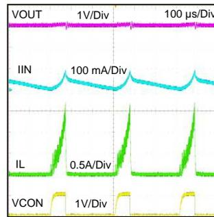
**Figure 37. Hiccup behavior with persistent output short circuit.**
