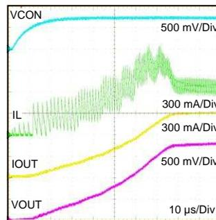
**Figure 36. Startup behavior of current limit based softstart.**
